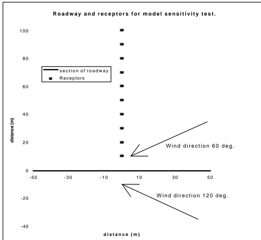
**Figure 3.22 Roadway and receptor configuration for the CAL3QHC sensitivity test showing wind direction vectors**
