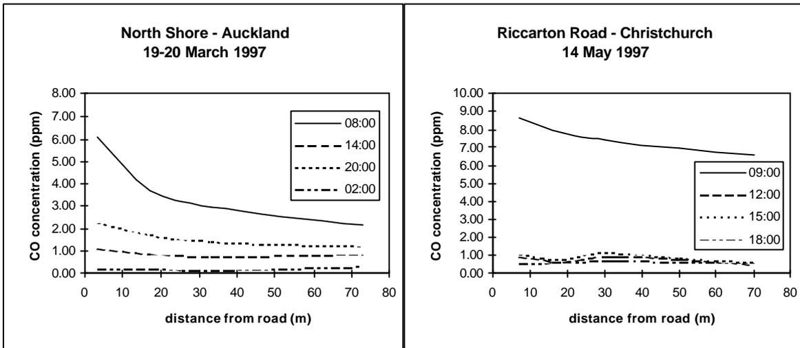
**Figure 3.7 Monitored carbon monoxide concentration change vs distance for (a) North Shore example (b) Riccarton Road example**
