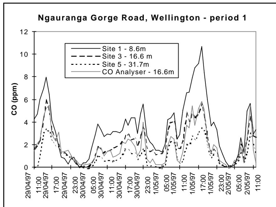
**Figure 3.4 Carbon monoxide measurements for Ngauranga Gorge Period 1 showing the pronounced afternoon peaks**
