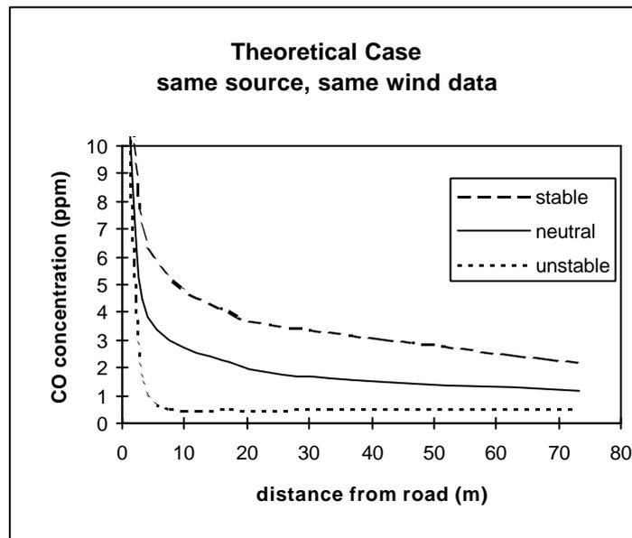
**Figure 3.8 Theoretical carbon monoxide concentration change vs distance for the same source and wind data showing the effect of stability**
