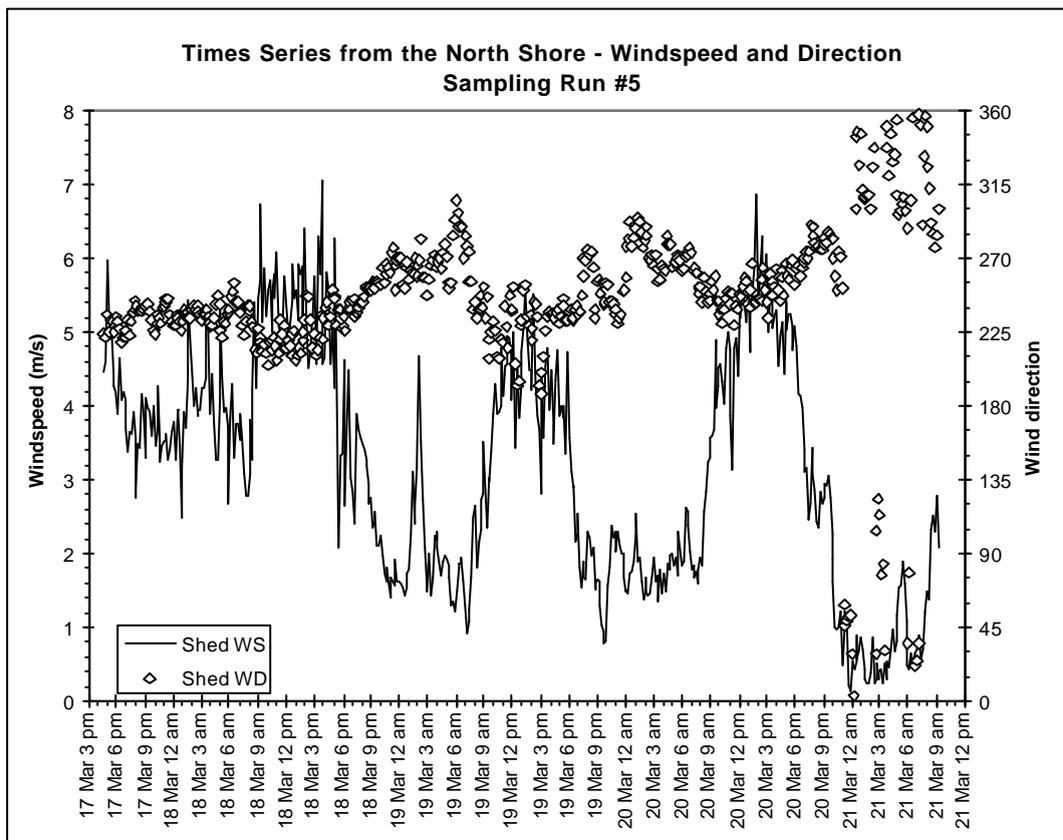
**Figure 3.1 Wind speed and wind direction for North Shore Period 5 showing a consistent westerly trend (note for wind direction: 360°=N, 270°=W, 180°=S, 90°=E)**
