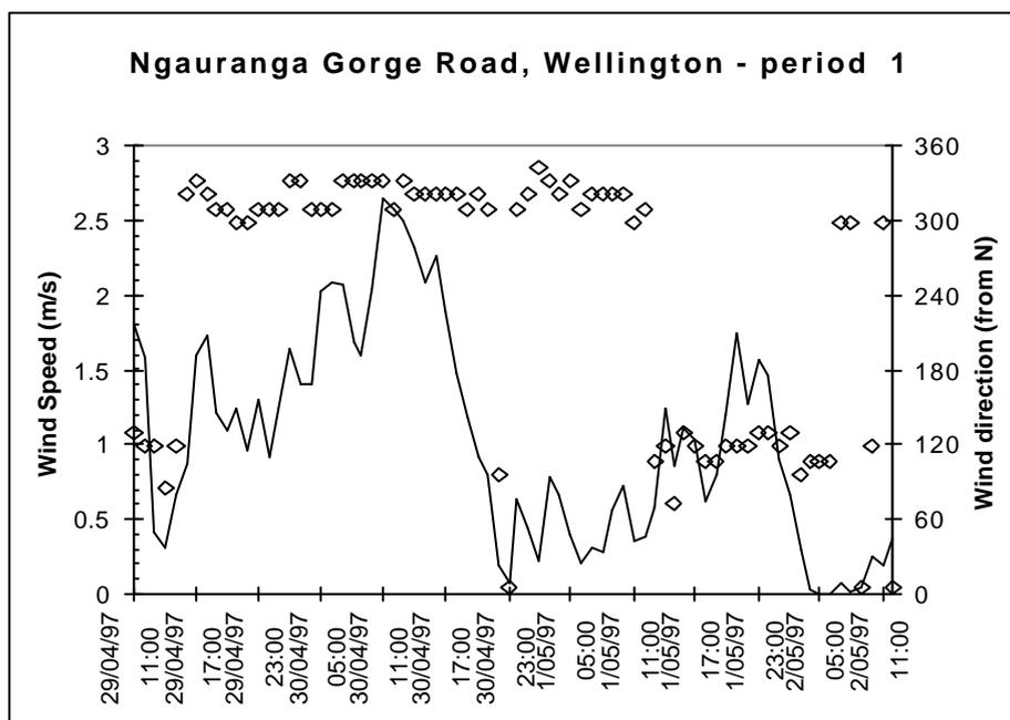
**Figure 3.3 Wind speed and wind direction for Ngauranga Gorge Period 1 showing wind-channelling in direction but a reduced diurnal pattern in speed (note for wind direction:  $360^\circ=N$ ,  $270^\circ=W$ ,  $180^\circ=S$ ,  $90^\circ=E$ )**
