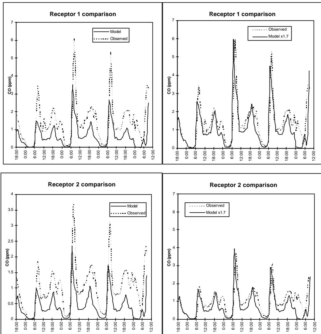
**Figure 3.24 Comparison of the modelled to the observed results for the original numbers (left) versus the scaled-up numbers (right) for receptors 1 and 2 in the Auckland case**
