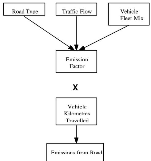
**Figure 0.2 Determination of road emissions**
