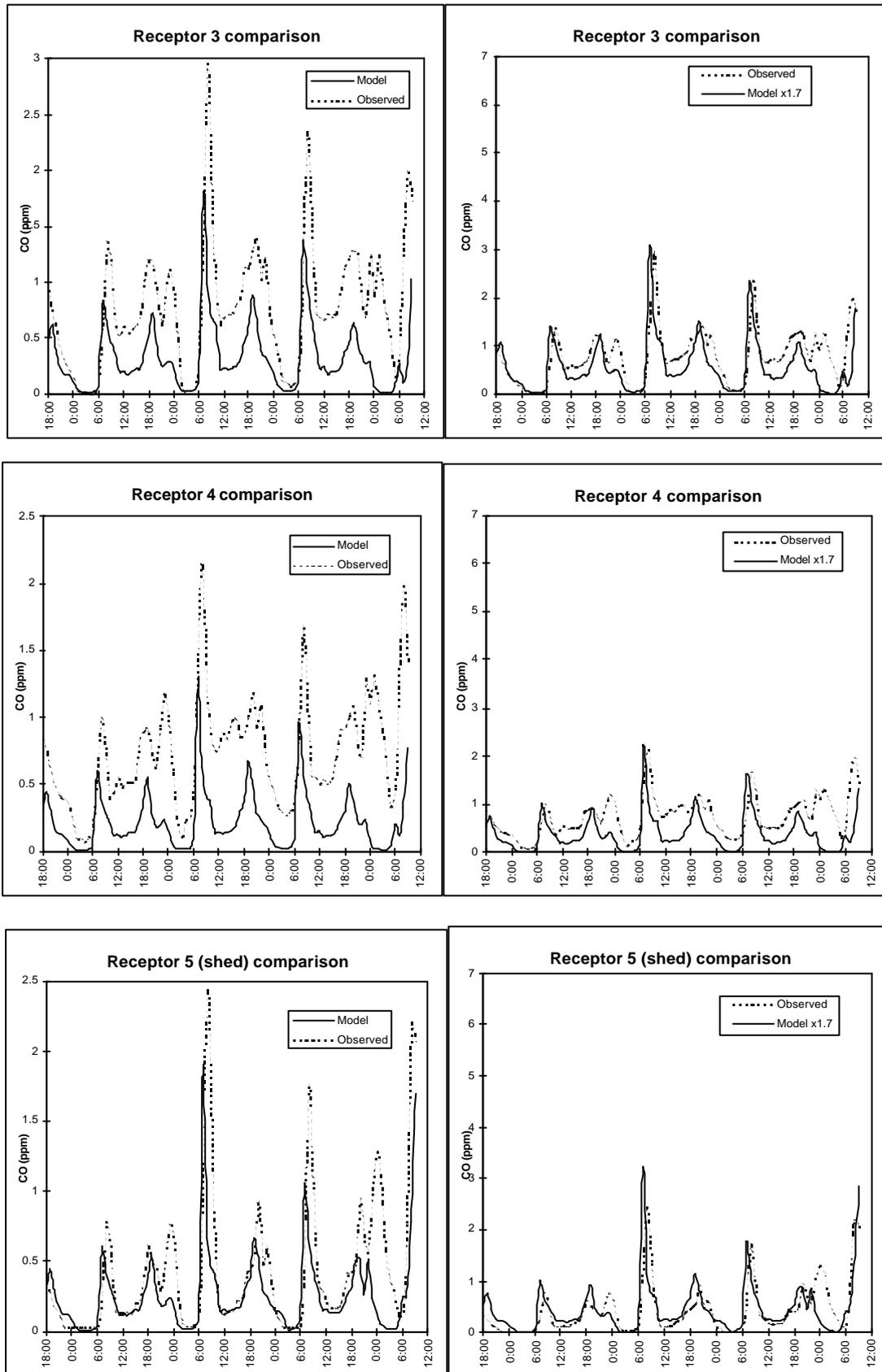
**Figure 3.25 Comparison of the modelled to the observed results for the original numbers (left) versus the scaled-up numbers (right) for receptors 3, 4, and 5 in the Auckland case**
