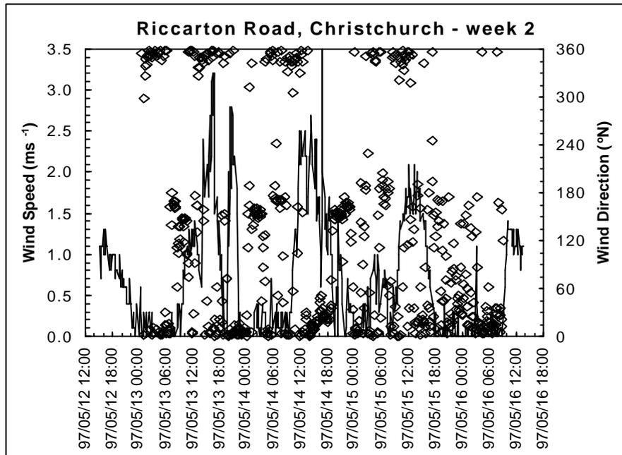
**Figure 3.5 Wind speed and wind direction for Riccarton Road Week 2 showing calm nights and light winds during the day (note for wind direction: 360°=N, 270°=W, 180°=S, 90°=E)**
