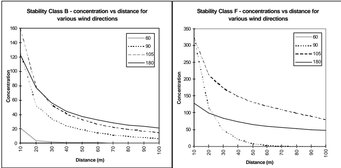
**Figure 3.23 Sensitivity of CAL3QHC to wind direction and stability class**
