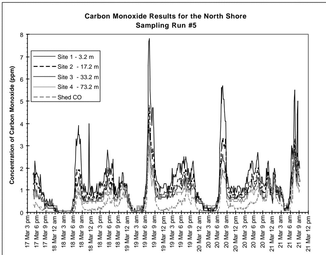
**Figure 3.2 Carbon monoxide measurements for North Shore Period 5 showing the daily trend of sharp morning and broad afternoon peaks**
