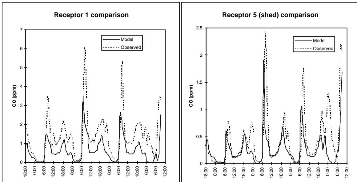
**Figure 3.13 Comparison between modelled and observed results for the Auckland case**
