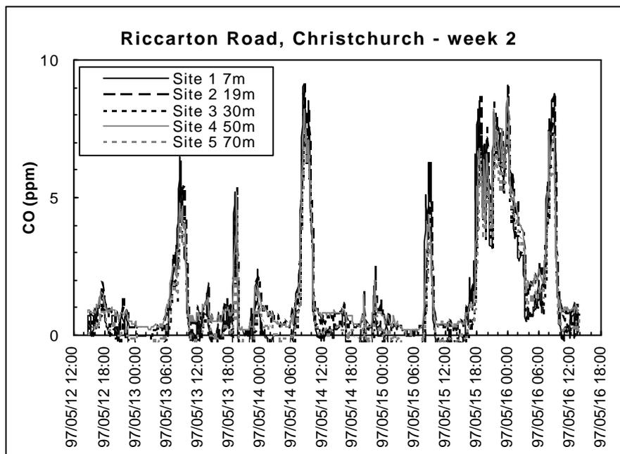
**Figure 3.6 Carbon monoxide measurements for Riccarton Road Week 2 showing the effect of traffic and wind speed on the peaks**
