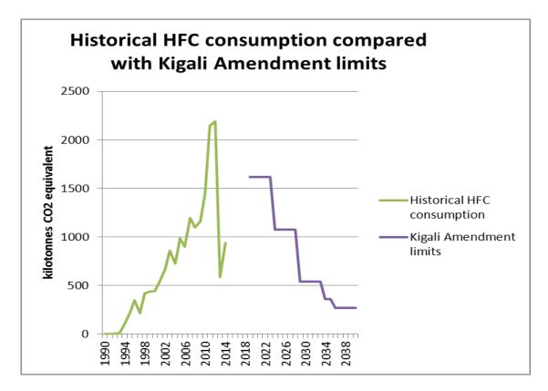
Bulk refrigerant R134a was the first HFC to be imported into New Zealand in 1992 as a major equipment manufacturer began to shift its production of commercial coolers and freezers from HCFC-22 refrigerant to R134a.
