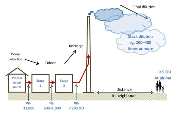
Figure 4: Industry/odour treatment schematic example: sewage treatment plant
