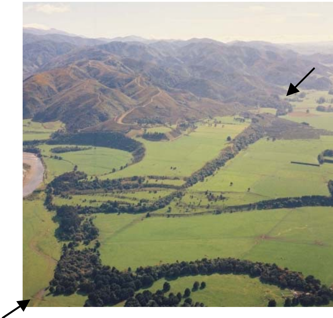
Figure 7.1: Wairarapa Fault – repeated rupture on same fault
