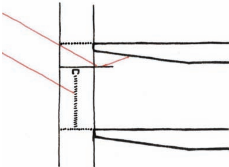
Figure 10: Shading strategies within a double skin facade; automated blinds are hung between the two glazing skins
