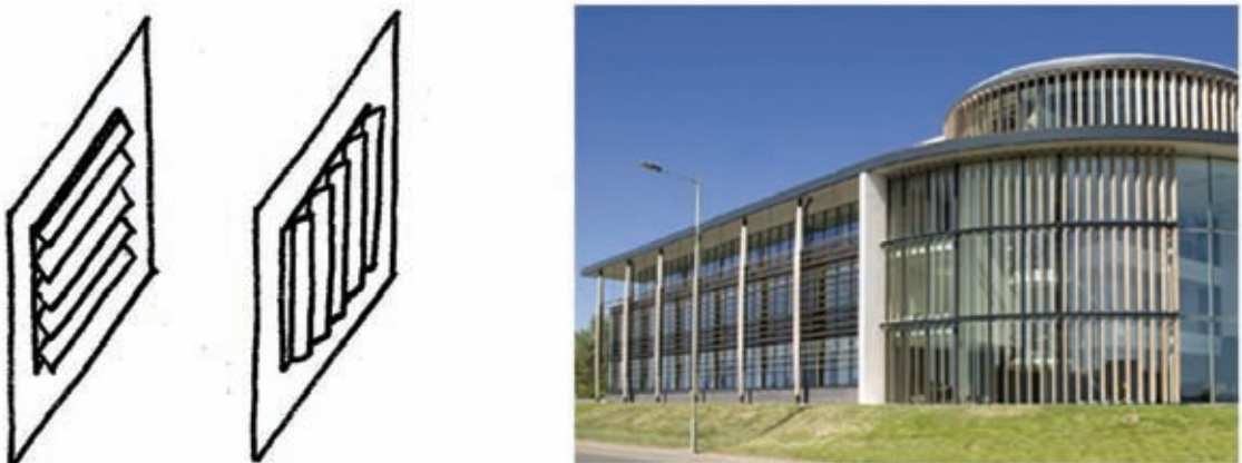
Figure 8: Horizontal and vertical louvres
