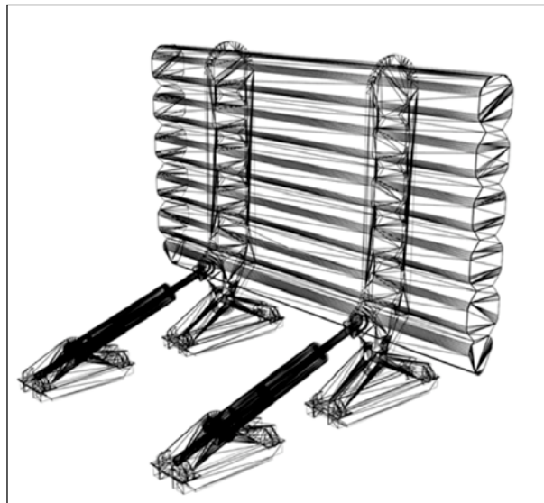
Figure 2.5: Aquamarine's Oyster Surge Device Design
