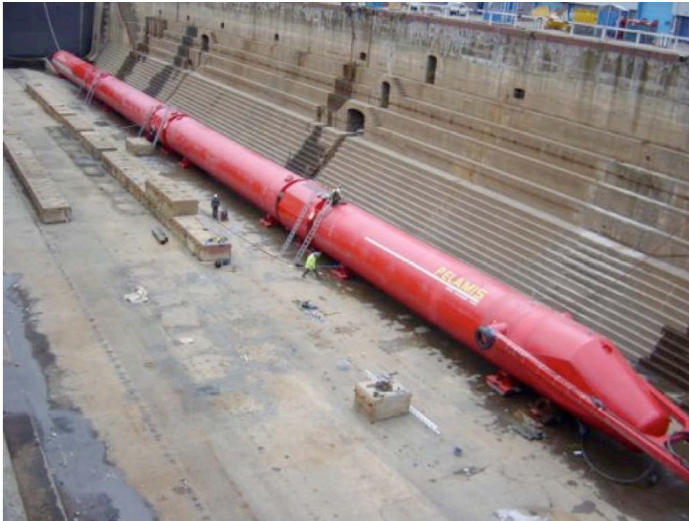
Figure 2.6: The Pelamis P750 Prototype in Leith, Edinburgh (workers show scale)
