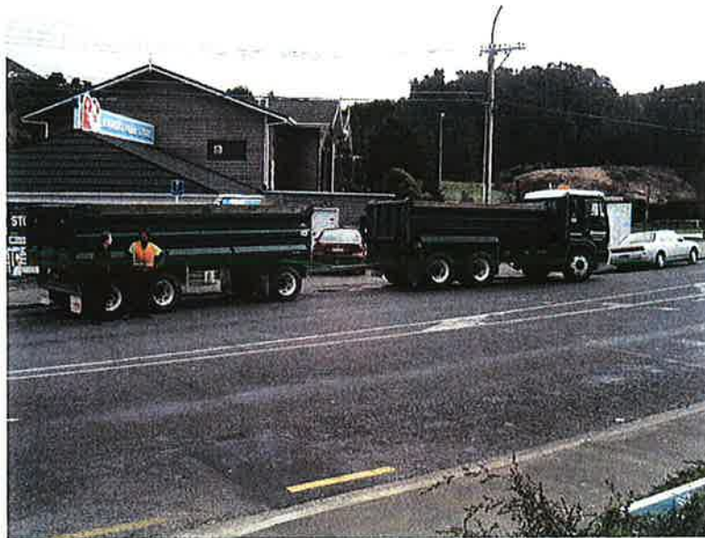
Photograph 2 : Typical truck and trailer unit for carting pavement materials
