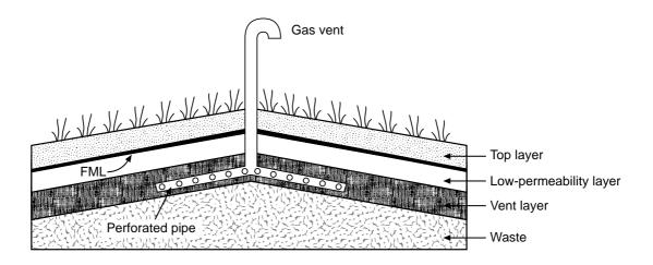
Figure 4.5 Example of passive landfill gas venting system (Figure 3-4 from USEPA Solid Waste Disposal Facility Criteria Technical Manual (1993))
