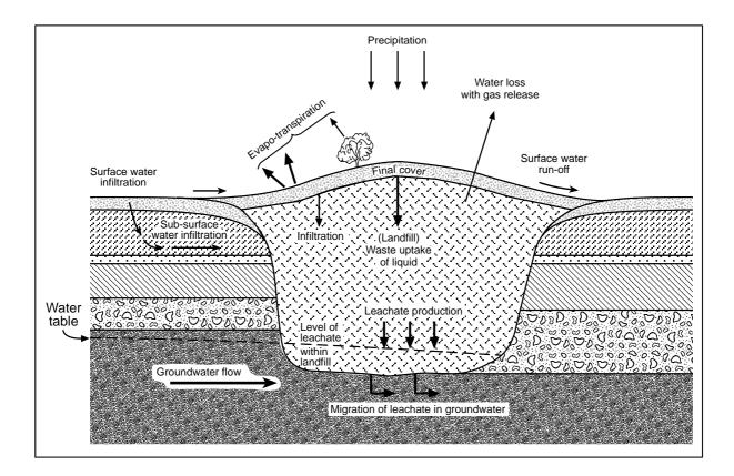
Figure 4.2 Landfill water balance issues (Figure 3.3 from UK Department of the Environment Waste Management Paper No. 26 (1986))
