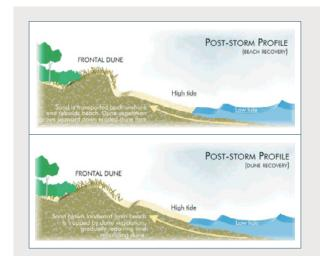
**Figure 2:** Typical response of a natural sand beachdune system to erosion during a storm, and how the beach and dunes build up again over the following months (and even years).
