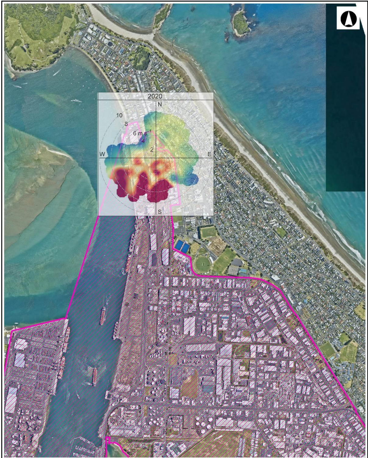
Figure 5. The Rata Street 2020 polar plot overlaid on aerial imagery to show source locations.
